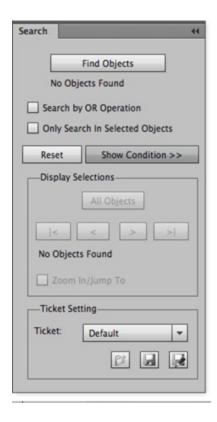
**4.** In the **Display Selections** section, the **All Objects** button selects all objects located by the search result. Use the arrows to navigate to the first. last, previous, or next object.
